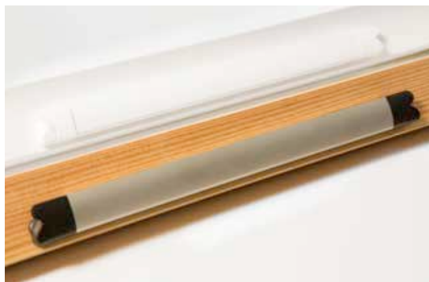
TRICKLE VENTS Equivalent areas 2500mm 2 , 4300mm 2 , 5000mm 2 and 8600mm 2 . Acoustic vents also available. (SAA finish)
